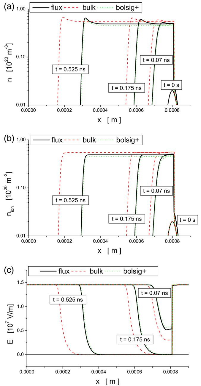
**Figure 6.** Temporal evolution of (a) the electron density, (b) the ion density and (c) the electric field in a planar negative ionization front in  $N_2$  with a reduced electric field  $E/n_0$  of 590 Td ahead of the front. Displayed are the spatial profiles obtained with three different sets of input data as indicated in the graph.
