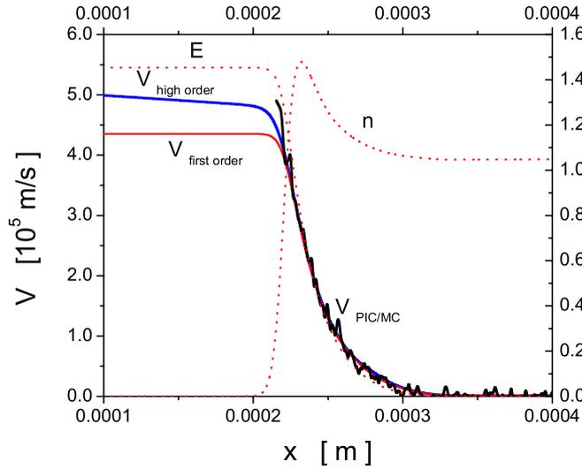
**Figure 5.** Profiles of the average electron velocity in the first- and the high-order fluid models and of the PIC/MC model at time 0.7 ns. Profiles of the electric field and of the electron number density from the first-order model are also included to indicate the location of the front. Calculations are performed for  $E/n_0$  of 590 Td. We remark that all velocities are negative, and their absolute value is plotted.
