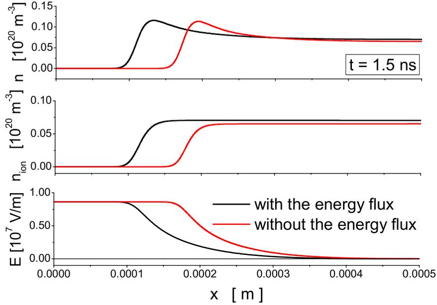
**Figure 8.** Electron density, ion density and electric field in  $N_2$  in an external electric field of 350 Td. The two lines indicate solutions of the high-order fluid model with and without the energy flux term at the same instance of time. The initial condition is the same, and the flux transport data are used.
