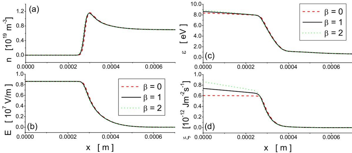
**Figure 11.** Profiles of (a) electron density, (b) electric field, (c) average electron energy and (d) average electron energy flux for  $\beta = 1$ ,  $\beta = 2$  and  $\beta = 3$ . The results are shown for  $E/n_0$  of 350 Td at time 1.5 ns.
