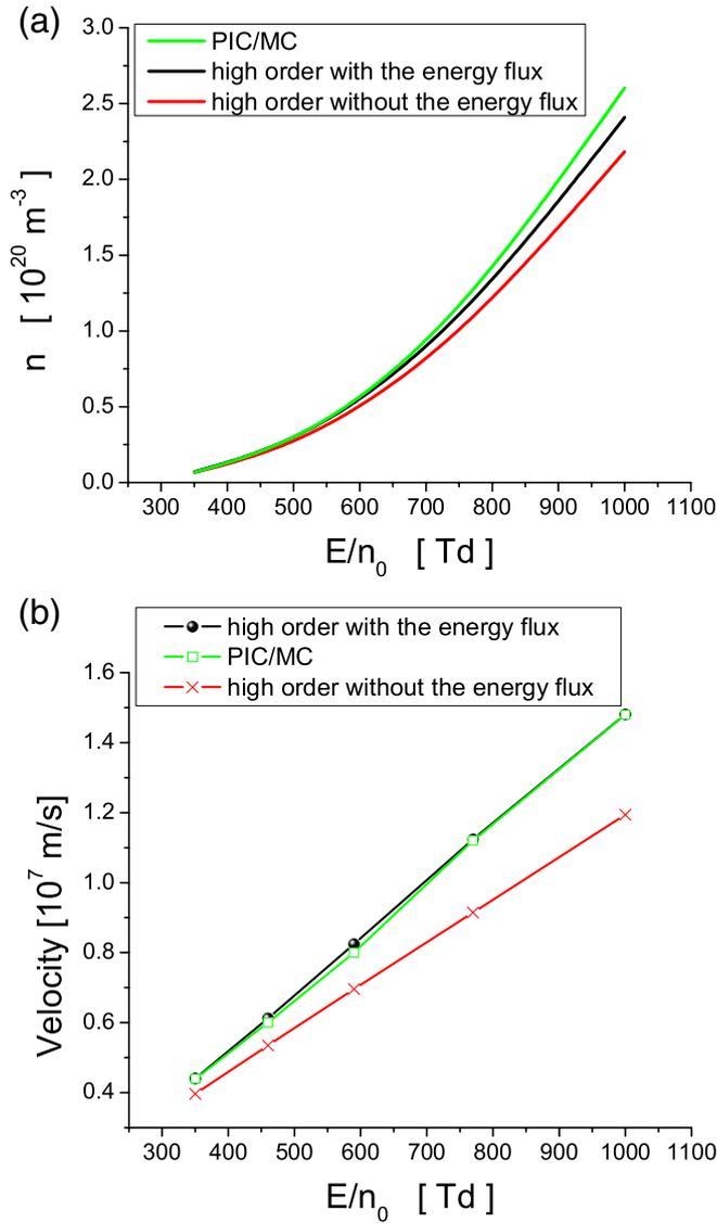
**Figure 10.** (a) Ionization level behind the planar front, and (b) the absolute value of the front velocity as a function of the reduced electric field  $E/n_0$  ahead of the front. Results are shown for the high-order fluid model with or without the energy flux term, as well as for the PIC/MC model. Flux transport data are used as an input in the fluid models.
