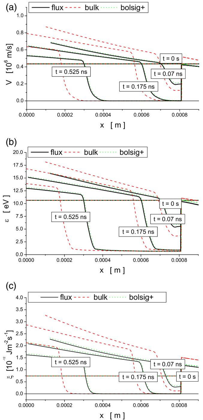
**Figure 7.** The same simulations and plots as in the previous figure, but now for (a) the average electron velocity  $v$ , (b) the average electron energy  $\epsilon$  and (c) the average electron energy flux  $\xi$ . Again, velocity  $v$  and energy flux  $\xi$  here are negative quantities, and their absolute value is plotted.
