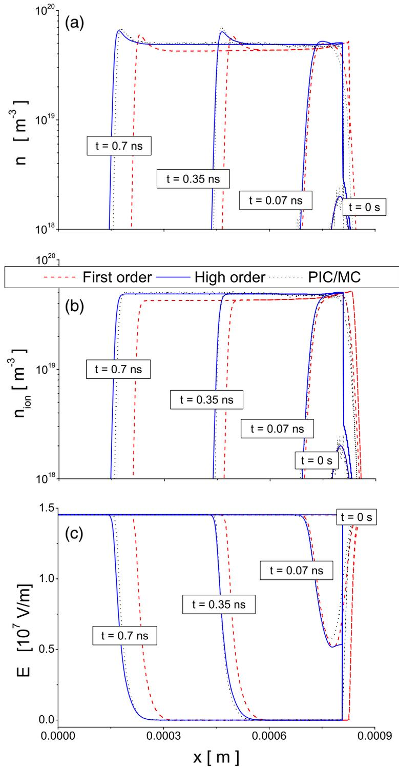
**Figure 1.** Temporal evolution of the electron density (a), ion density (b) and electric field (c) in a planar front in  $N_2$ . Shown are the spatial profiles obtained with three different models as indicated on the graph. Flux transport data are used as an input in fluid models. The externally applied reduced electric field is 590 Td.
