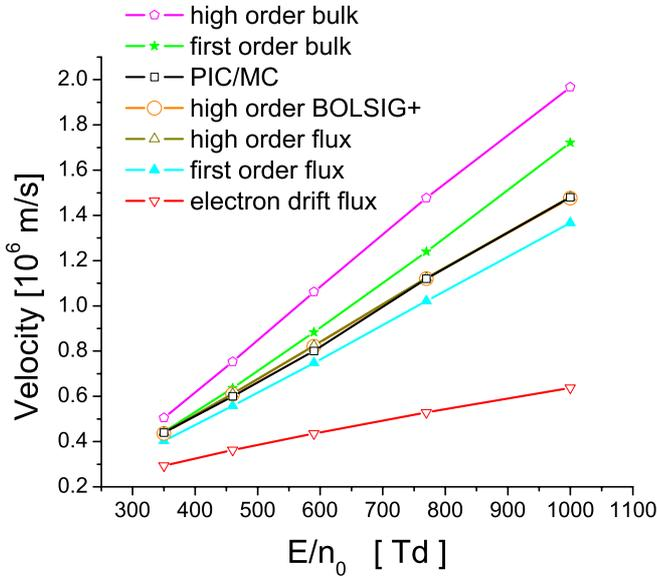
**Figure 2.** Velocities of planar fronts as a function of the electric field obtained with the first- and the high-order fluid models and with the PIC/MC method; different sets of input data are used as indicated on the graph. The electron flux drift velocity as a function of  $E/n_0$  is also included. We remark that the negative sign of all velocities is removed here.
